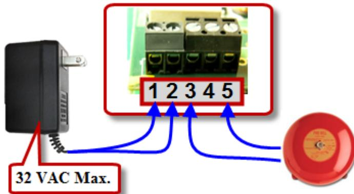
1. Plug the AC line of the external power source on pin 1 of JP1.
