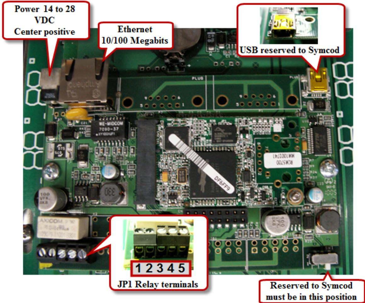
The output relays (JPI connector) offer a dry contact either normally closed or normally opened. The relay allows the activation or de-activation of a door strike or a door magnet but **it does not provide power to either the door strike nor to the door magnet**. The input voltage should never exceed 32 volts AC or DC.
