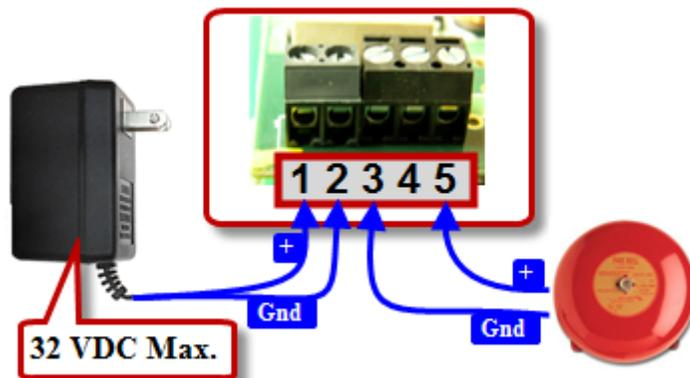
1. Plug the positive of the external power source on pin 1 of JP1.
