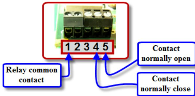
Terminal 2 and 3 are electrically connected together.
