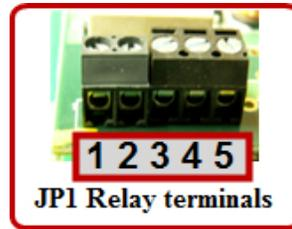
The output relay (JP1 connector) offer a dry contact either normally closed or normally opened. The relay allows the activation or de-activation of a bell, but **it does not provide power**. The input voltage should never exceed 32 volts AC or DC 4 Amps resistive.
